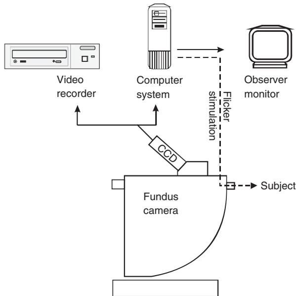
**Fig. 2.** Schematic view of the retinal vessel analyzer/dynamic vessel analyzer system. CCD, charge-coupled device.
