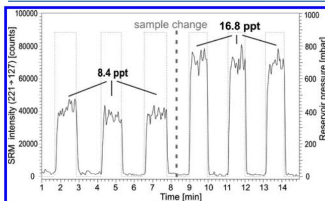
**Figure 2.** DBDI SRM signal ( $221\text{ m/z} \rightarrow 127\text{ m/z}$ ) for three consecutive generations of two different dichlorvos gas phase concentrations (8.4 and 16.8 ppt) (solid line). The dotted line shows the pressure applied to the nanospray sample reservoir (right y-axis).
