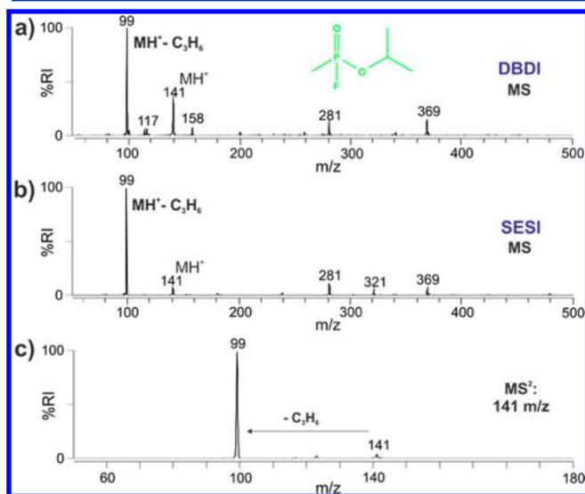
**Figure 4.** MS and MS/MS (c) spectra and molecular structures (green) for a concentration of 500 ppt Sarin (GB) acquired with DBDI (a) and SESI (b). Spray voltage was 2.7 kV for SESI, and DBDI voltage amplitude was 1.6 kV p-p. Isolation window width for MS<sup>2</sup> experiments was 1.0  $m/z$ .
