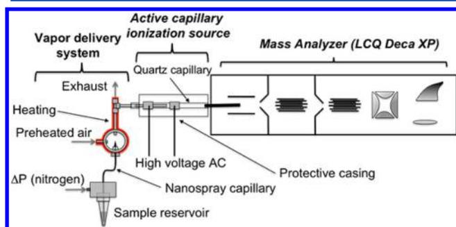
**Figure 1.** Schematic drawing of the system setup, including the vapor delivery system for the generation of ppt gas phase concentrations, the active capillary ionization source, and a scheme of the LCQ Deca XP mass analyzer. (Note: Not to scale for better representation.)
