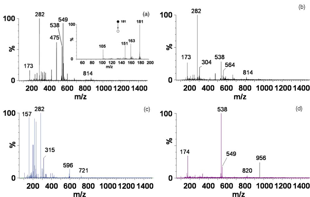
**Figure 10.** Extractive electrospray ionization mass spectral fingerprints recorded from the same volunteer but different skin areas during *in vivo* skin analysis: (a) fingerprints recorded from the forehead skin. The inset shows the CID spectrum of a peak at  $m/z$  181, which is identified as due to protonated glucose; (b) fingerprint obtained from abdominal skin; (c) fingerprint obtained from the forearm skin; (d) fingerprint obtained from the foot skin.
