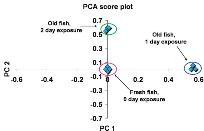
**Figure 3.** Score plots of principal component analysis of the full set of mass spectral data obtained from fish meat at different stages. Each cluster contains five points referring to five desorption EESI-MS spectra obtained from five fish cuts.
