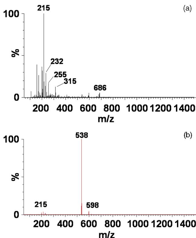
**Figure 11.** Extractive electrospray ionization mass spectral fingerprints obtained from the same skin area but different desorption reagents: (a) nitrogen as desorption gas; (b) nitrogen and acetone vapor as desorption gas.
