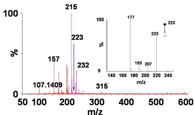
**Figure 12.** *In vivo* detection of explosive contaminant RDX in a skin sample. Protonated RDX ( $m/z$  223) is detected in a forearm skin exposed to RDX contaminated air; the inset shows the CID spectrum of the peak at  $m/z$  223.
