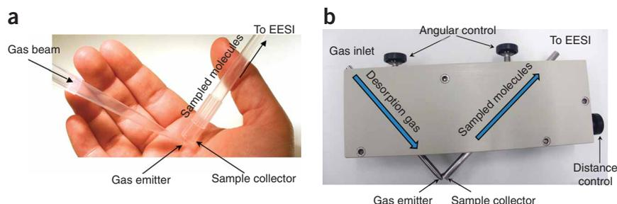
**Figure 1** | Photographs of ND-EESI sampling devices. (a) An easily available plastic ND device for *in vivo* sampling of hand skin, consisting of a pipette tip as a gas nozzle and a plastic sleeve connected to a plastic tubing for collection of the desorbed material. (b) Adjustable gas emitter/collector device fabricated from stainless steel, with better control of the operating parameters.
