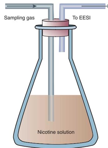
**Figure 4 |** Setup for introduction of nicotine as a standard compound for the optimization of EESI.
