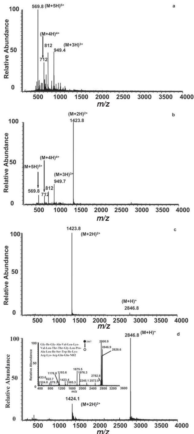
Figure 3. Dynamic charge states of melittin; (a) high charge states generated in ESI; (b) intensity of multiply charged ions decreased by spraying a small amount of neutral base into the electrospray beam; (c) doubly charged ions generated exclusively by the ion/molecule reactions; (d) singly charged ions generated by the ion/molecule reactions in open air.
