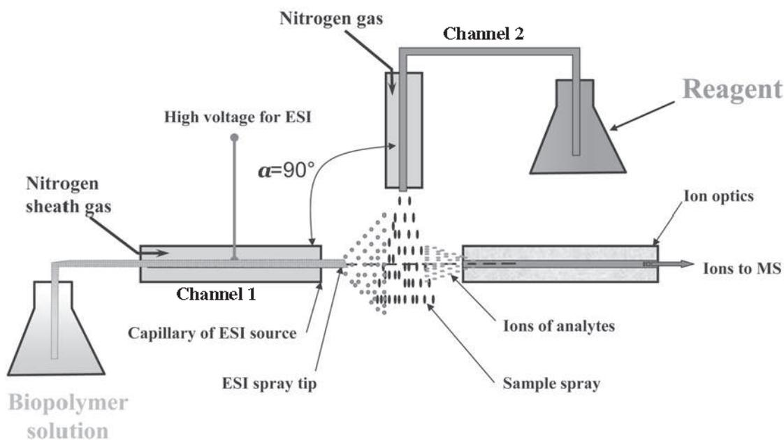
Figure 1. Schematic diagram of the EESI source used for ion/molecule reactions at ambient conditions.
