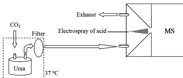
Fig. 1. Experimental set-up used to detect urea vapors.
