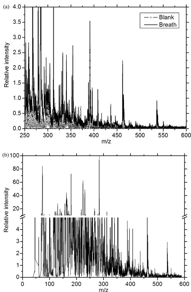
Fig. 2. ESI spectra from one subject's breath, from [5]. (a) (Top), breath and blank (clean CO<sub>2</sub>). (b) (Bottom), breath spectra after subtracting the blank.
