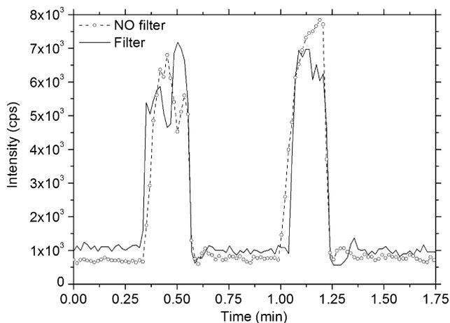
Fig. 5. Total ion current spectrum at 445 Da, breathing with and without filter in the line.
