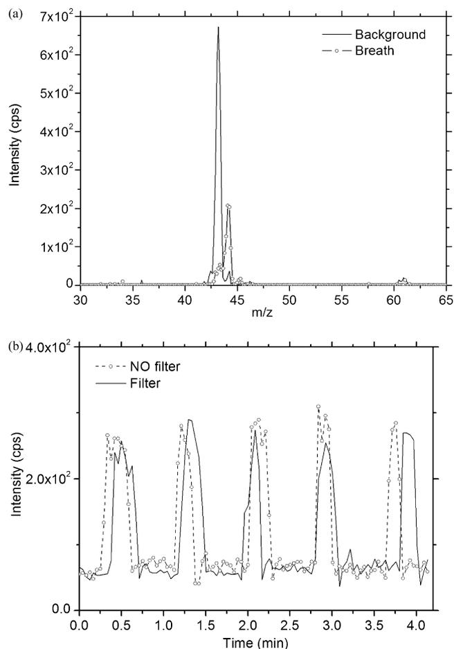
Fig. 3. Analysis of urea vapors in breath, with the first quadrupole fixed at 61.1 Da. (a) (Top), fragmentation spectrum showing the presence of a background peak with a characteristic fragment at 43 Da, mixed with breath urea, with a characteristic fragment at 44 Da (protonated urea-NH<sub>3</sub>). (b) (Bottom), total urea ion current spectrum at 44 Da, from filtered and unfiltered breath.
