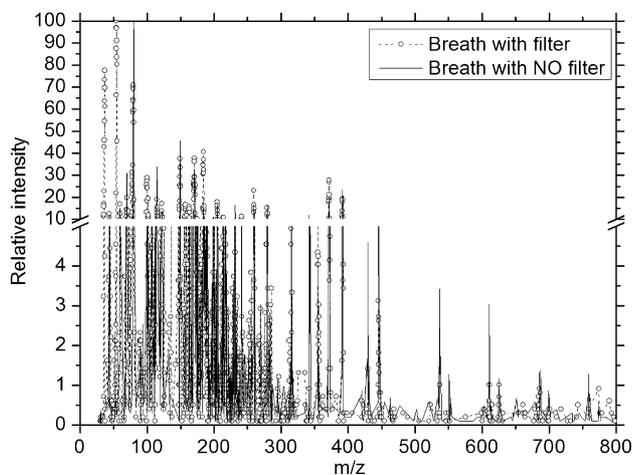
Fig. 4. Mass spectrum of a subject's breath, either blowing directly to the MS, or going first through a filter. Even the highest molecular weight peaks survive through the filter.
