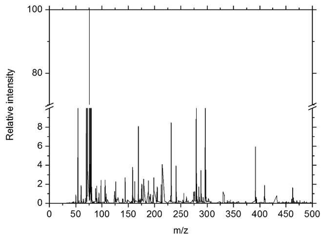
Fig. 6. Breath mass spectrum obtained after subtracting ambient air background in a protocol (discussed in Section 2.4) which preserves exactly the charging probability of the breath and the background.
