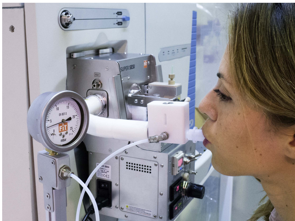
Figure 4. Complete system enabling real-time breath analysis by SESI-HRMS in a standardized fashion. The exhalation pressure is monitored with an analog manometer. In addition, the regulator features a variable opening that further stabilizes the pressure and the flow passed into the analyzer. This flow matches the optimal one found by the numerical simulations (figure 2).
