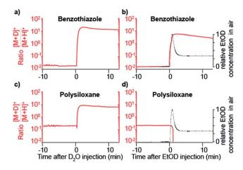
**Fig. 3** Gas-phase proton affinity of seeding vapors have an effect in SESI analyte detection. Benzothiazole deuterates after adding vapors of  $D_2O$  (a) and EtOD (b) in the carrier gas. In contrast, the deuterated form of the polysiloxane was detected with  $D_2O$  (c), but depleted upon exposure to EtOD vapors (d). Relative concentrations of EtOD in the carrier gas are shown for reference.
