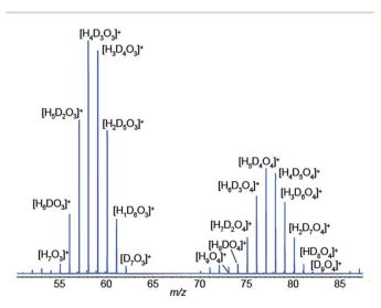
**Fig. 5** SESI gas-phase reactant ions in the presence of humidity are water clusters. Example of an electrospray of 0.15% formic acid in water flushed with a 50/50 mixture of  $H_2O/D_2O$  vapors, leading to all possible  $[H_xD_yO_3]^+(x + y = 7)$  combinations for the trimer (left-hand-side) and  $[H_yD_yO_4]^+(x + y = 9)$  for the tetramer (right-hand-side).
