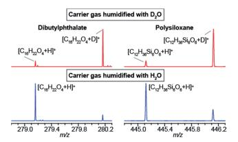
Fig. 2 Humidifiying the carrier air with deuterated water leads to deuterated ions in SESI-MS. Electrospray solvent was 0.15% formic acid in H<sub>2</sub>O. Mass spectra of dibutylphthalate (left) and a polysiloxane (right). As expected, humidifying with H<sub>2</sub>O leads to protonated species (i.e.  $[M + H]^+$ ; bottom) and humidifying with D<sub>2</sub>O leads to deuterated species (*i.e.*  $[M + D]^+$ ; top)
