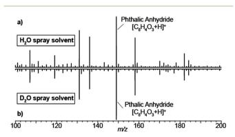
Fig. 1 SESI mass spectra are independent of whether electrospray solvent is water or deuterated water. SESI chemical noise mass spectra with different electrospray solutions: (a) 0.15% formic acid in  $H_2O$ ; (b) 0.15% deuterated acetic in D<sub>2</sub>O. In both cases, the analytes were detected in protonated form. For reference, the dominating peak of phthalic anhydride is labelled.
