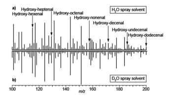
Fig. 6 Breath metabolites are ultimately protonated *via* gas-phase ion-molecule reactions in SESI: (a) breath mass spectrum using 0.15% formic acid in water; (b) breath mass spectrum using 0.15% acetic acid-d<sub>4</sub> in heavy water. Breath metabolites were detected in protonated form regardless of the solvent used to generate the electrospray. For reference, a series of hydroxy-alkenals previously identified by García-Gómez<sup>63</sup> are indicated.
