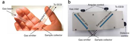
**Figure 1** | Photographs of ND-EESI sampling devices. (a) An easily available plastic ND device for *in vivo* sampling of hand skin, consisting of a pipette tip as a gas nozzle and a plastic sleeve connected to a plastic tubing for collection of the desorbed material. (b) Adjustable gas emitter/collector device fabricated from stainless steel, with better control of the operating parameters.
