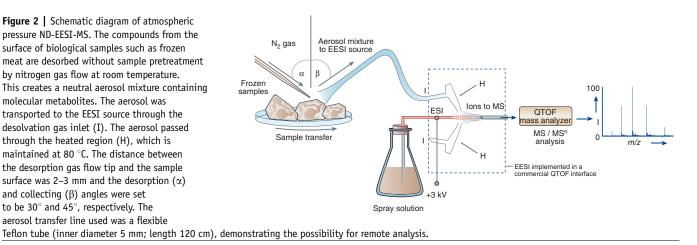
spectrum is recorded by the TOF analyzer. The sensitivity of EESI could be further improved if the EESI source could be precisely adjusted (e.g., with hardware modifications).
