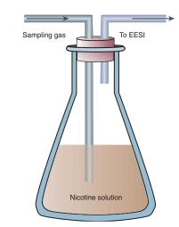
Figure 4 | Setup for introduction of nicotine as a standard compound for the optimization of EESI.
